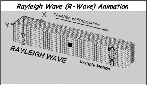
Deformation propagates. Particle motion consists of elliptical motions (generally retrograde elliptical) in the vertical plane and parallel to the direction of propagation. Amplitude decreases with depth. Material returns to its original shape after wave passes.
