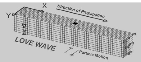
Deformation propagates. Particle motion consists of alternating transverse motions. Particle motion is horizontal and perpendicular to the direction of propagation (transverse). To aid in seeing that the particle motion is purely horizontal, focus on the Y axis (red line) as the wave propagates through it. Amplitude decreases with depth. Material returns to its original shape after wave passes.
