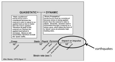
A stress wave transmits energy and momentum away from source of loading *without* bulk translation of mass, at a finite velocity in any given material
