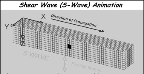
Deformation propagates. Particle motion consists of alternating transverse motion. Particle motion is perpendicular to the direction of propagation (transverse). Transverse particle motion shown here is vertical but can be in any direction. However, Earth's layers tend to cause mostly vertical (SV; in the vertical plane) or horizontal (SH) shear motions. Material returns to its original shape after wave passes.
