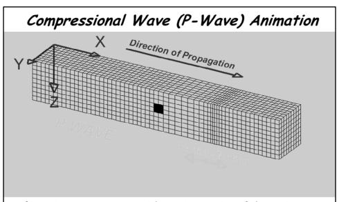
Deformation propagates. Particle motion consists of alternating compression and dilation. Particle motion is parallel to the direction of propagation (longitudinal). Material returns to its original shape after wave passes.
