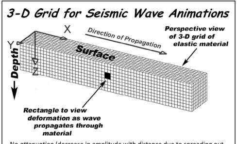
No attenuation (decrease in amplitude with distance due to spreading out of the waves or absorption of energy by the material) dispersion (variation in velocity with frequency), or anisotropy (velocity depends on direction of propagation) is included.
