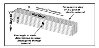
The mechanical description, and formulations for wave speed and interactions with boundaries relies on there being an atom or molecule at each intersection in the grid above, and that the gridlines are the forces associated with bonding.
