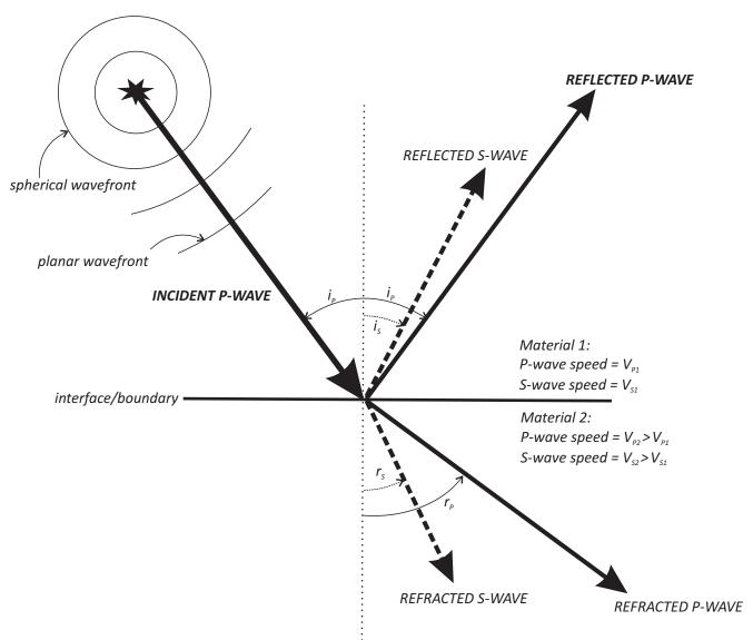
The dynamic stress traveling from a far-away source arrives at the boundary or interface between two distinct (but mechanically connected) materials with a planar wavefront; consider the 'ray path' (bold arrow) of the incident P-wavefront when it hits the boundary.
