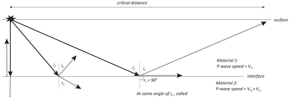
Normal incidence: wave is partially reflected, partially transmitted with no refraction - since  $i_p = 0$ , therefore  $r_p = 0$  (Snell's Law)
