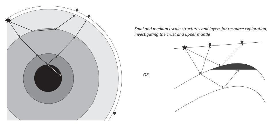
Seismological surveys are based on knowledge of how stress waves travel through different layers from a source of energy to the location of a seismometer. The geophysicist must solve for the unknown of interest (such as the depth to a layer, the properties of a layer, the source of the energy or earthquake).
