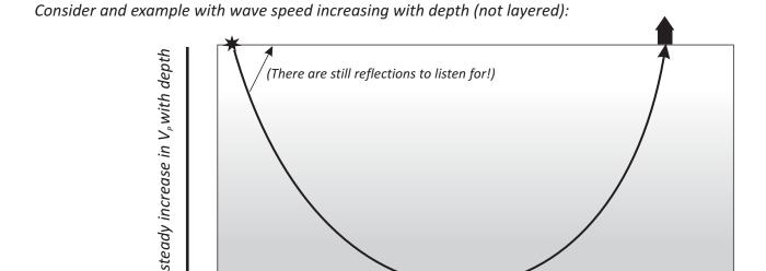
The wave refracts as if encountering many thin layers, and will eventually reach a critical angle and be reflected back toward the surface
