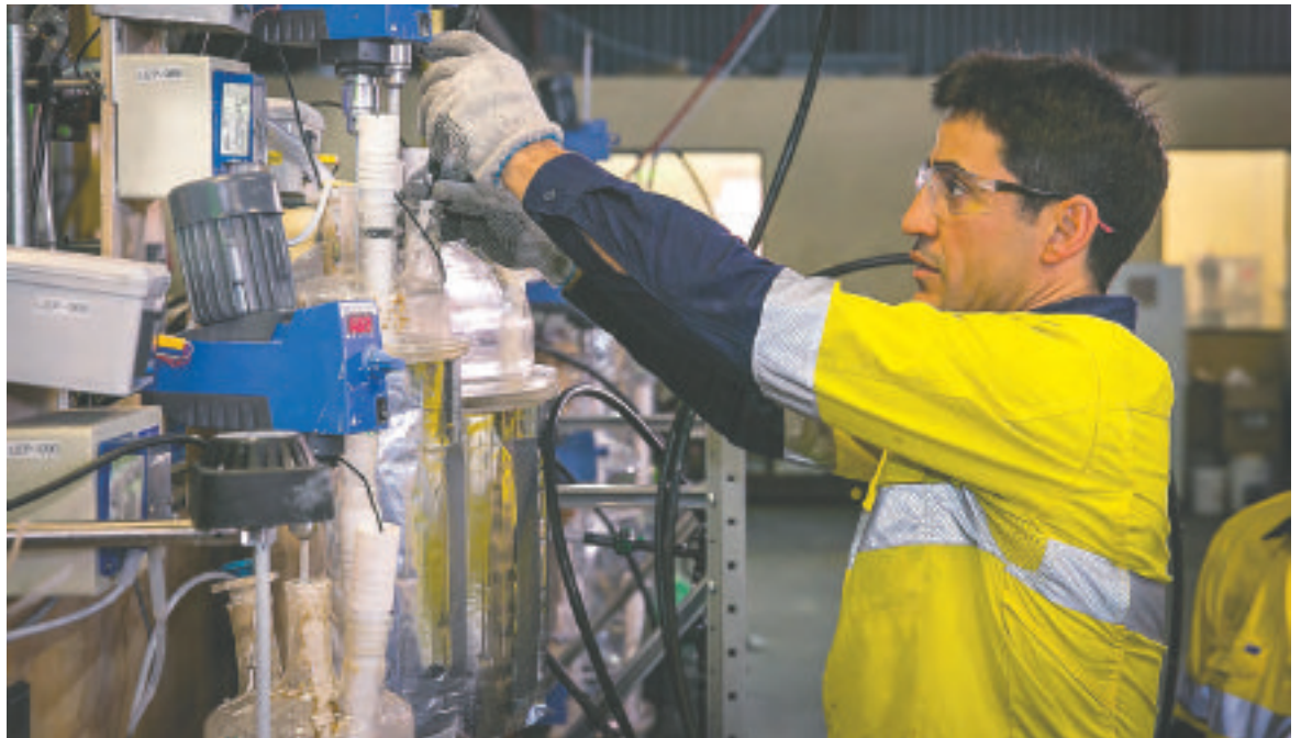
Mini plant run for the L-Max process in Australia produced a high-specification lithium carbonate product with a purity of 99.5 per cent.
