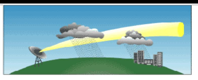
Effects of curvature of the Earth on weather radar
