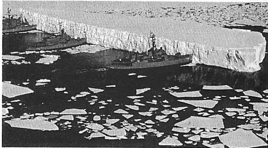
FIGURE 4.10 A tabular iceberg derived from an ice shelf being moved from the approaches to McMurdo Station, Antarctica, by three U.S. ice breakers in 1966. U.S. Navy photograph.
