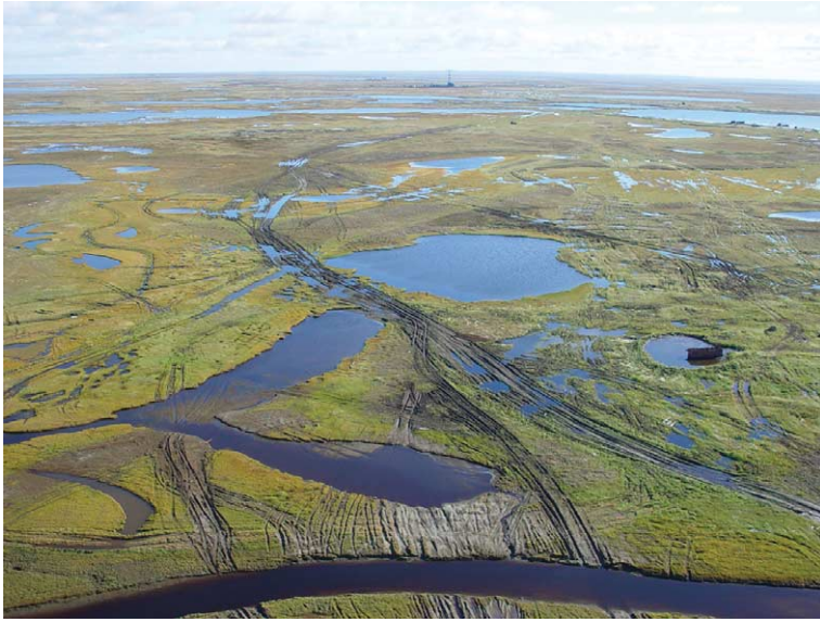
Figure 5. Pattern of cross-cutting vehicle tracks from driving on unfrozen ground in the Varandey area. Such activity causes considerable harm to the tundra soil and vegetation and is illegal in Russia. Photo: Yasavey, September 2002.
