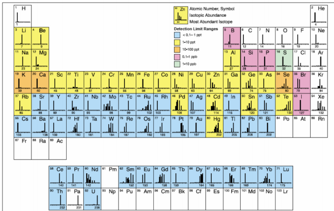
Figure 1: shows the detection limits for elements that can be measured by ICP-MS (Photo from Wolf, 2005 courtesy of Perkin Elmer Inc., 2001)
