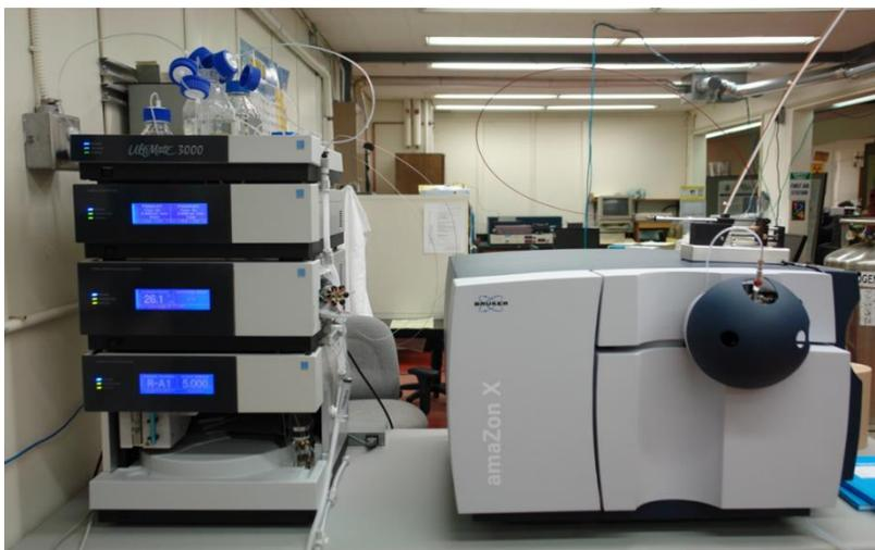
This new ion trap compliments the existing Gas Chromatograph – Mass Spectrometer (GC-MS) at Lakehead's Instrumentation Laboratory (LUIL). Users will no longer be limited to running only volatile samples with a maximum mass of 800amu. The new system can run a wide range of samples with a mass range of 50-3000amu, opening the door for proteomics and metabolite identification that was not previously possible on the GC-MS, as well as expanding the use for general chemistry.
