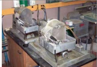
Powders are mixed with expoxy, then spread on a slide and allowed to cure. The surface is ground flat on the thin section grinder, then finished similarly to a thin sections
