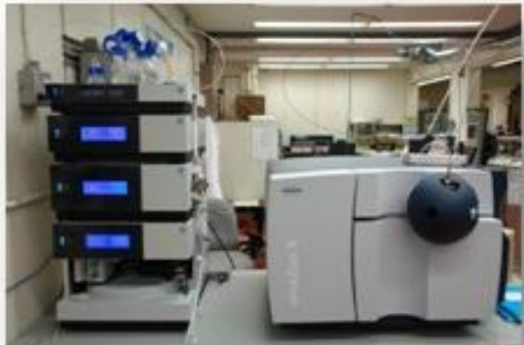
This new ion trap compliments the existing Gas Chromatograph – Mass Spectrometer (GC-MS) at Lakehead’s Instrumentation Laboratory (LUIL). Users will no longer be limited to running only volatile samples with a maximum mass of 800amu. The new system can run a wide range of samples with a mass range of 50-3000amu, opening the door for proteomics and metabolite identification that was not previously possible on the GC-MS, as well as expanding the use for general chemistry.
