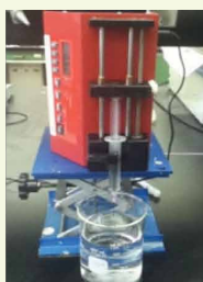
Gel extruded in acid bath
