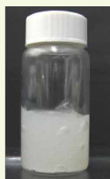
Gel prepared with chitosan
