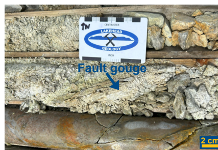
Fault gouge indicates incohesive brittle grain size reduction
